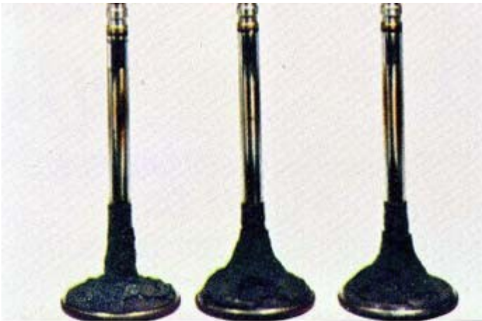
3,000 mile drain interval using conventional Petroleum Oil
