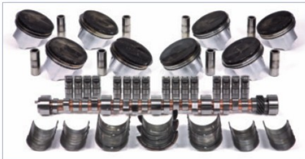
Bearings, camshaft, lifters and pistons from Mercury 525 EFI powerboat engine. Following teardown, Mercury technicians found the engine "extremely clean internally."
