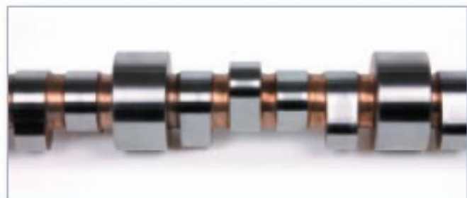
Camshaft shows no signs of wear or bluing.
