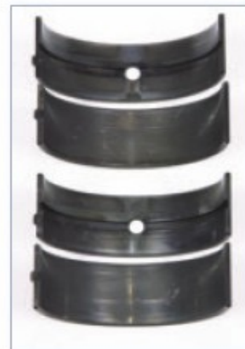
Close-up of main bearings. Notice absence of wear despite over 3,000 miles of use in racing applications.
