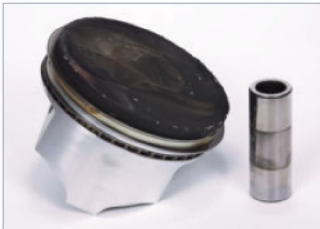
Piston from Team AMSOIL Mercury 525 EFI powerboat engine. Minimal carbon deposits on top of piston. Skirt clean with no scuffing.
